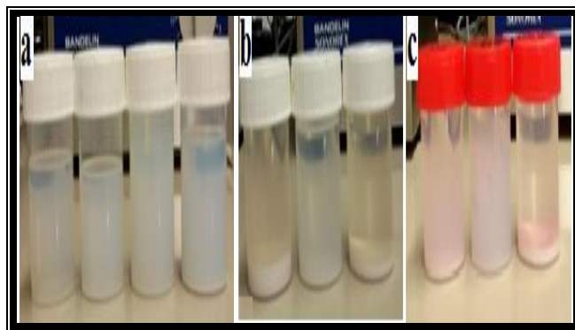
Figure 2: stabilization of suspension after preparation in a solution of. (a) Isopropanol, (b) ethanol–17% water, and (c) Ethanol.
