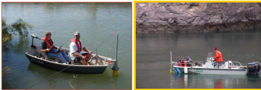
Figure 2: Discharge Measurement by RiverSurveyor ADP equipment (RiverSurveyor Manual, 2005)
