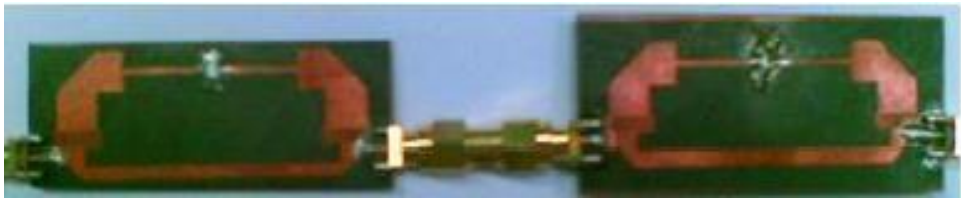
Fig. 1. Photograph of multiband bandstop filter design
