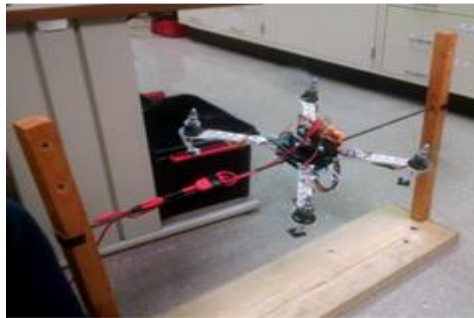
Fig 4. Quadcopter Three-Axes Test Stand
