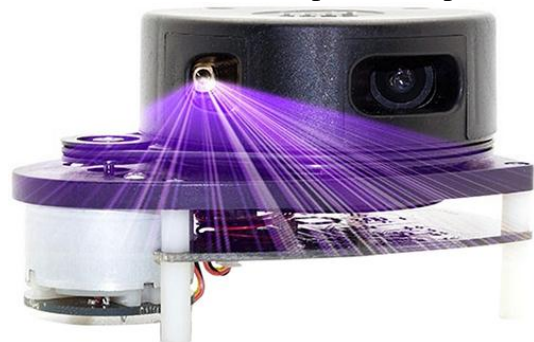
Fig 2. Leaser scanning device
